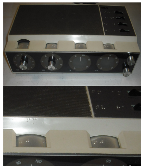
Above: RCA AM, FM, UHF-TV, VHF-TV receiver with braille-character dial references.
