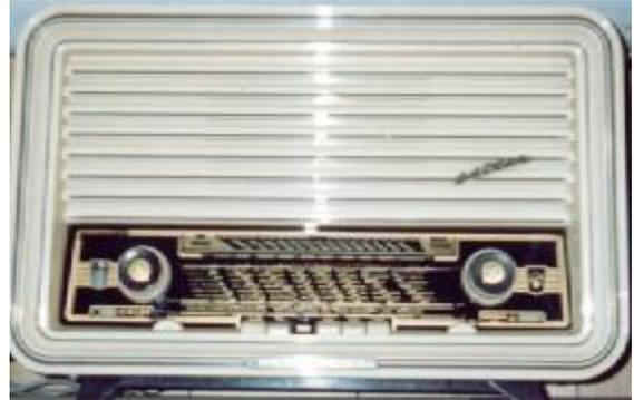
Like many German sets the Sultan uses a "matchbook" selenium rectifier. Replace it with a silicon bridge plus a 30-40 ohm 10 watt series resistor.
