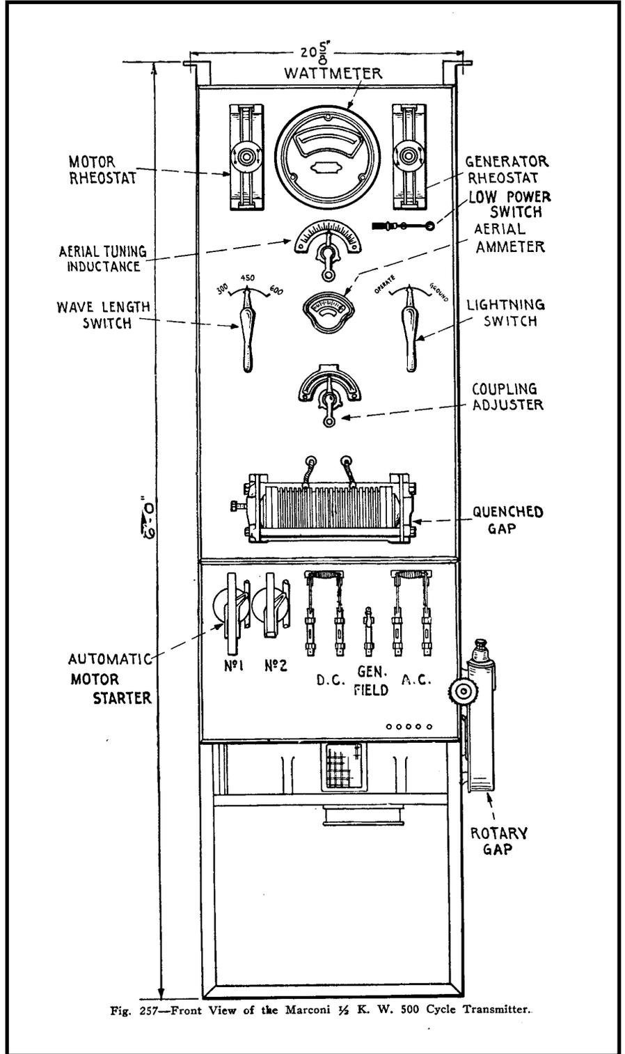
Fig. 257—Front View of the Marconi 1/4 K. W. 500 Cycle Transmitter.
