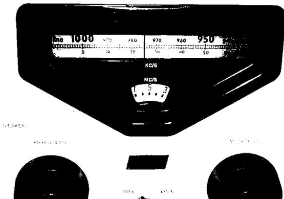
The "KILOCYCLES" knob controls the best part of the receiver, a 6-foot piece of 35mm film that serves as the kilocycle readout. It has about 20 1-KHz divisions per inch. The manual proudly points out that the 0.5 to 30-MHz tuning range is effectively spread across 145 feet! The RA.17 is my pick for the best SWL "band cruiser" of all time, offering the smooth unencumbered tuning of a high-end Hammarlund and the frequency accuracy associate with the Collins products.
