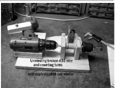
Clear tape and cement held the fine number 36 wire in place as the coil was rewound. The set played quite nicely with the repaired transformer in place. Hooray!!
