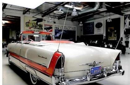
Above: This 56 Packard came from factory with dual antennas. 55-56 Caribbeans had them and since it balanced the appearance, they put them on other Packard models. Both antennas are powered but only the one on the right side was connected to the radio originally.
