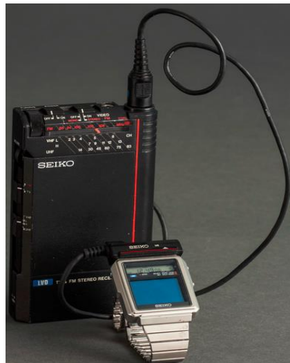
The Guinness Book of Records showed, in its 1984 edition, the SEIKO TV-Watch as the "smallest TV set in the world". This is an interesting theory, since from what you can see here actually looks like the smallest TV by far. Unfortunately, a vital detail is missing; the necessary TV receiver is inside a box about the size of a Walkman.
