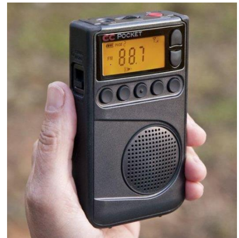
Above and Below: Jarret Brown showed a CC Crane Pocket radio made by CC Crane. Jarret uses this one the most of all his radios listening at night or taking outside. Features sleep timer (no auto shut-off), clock and alarm and removable belt clip. Five memory pages for AM/FM, 50 memories total. 1, 9 or 10 KHz selectable tuning steps. Selectable Narrow or Wide AM filter. LCD shut off to reduce radio noise. NOAA Weather Radio with Alert (disables AM/FM radio while activated). Rubber protected sides. Runs on (2) "AA" batteries. About 75 hours of play with earphones, 25 hours using built-in speaker. Excellent selectivity with maximum sensitivity.
