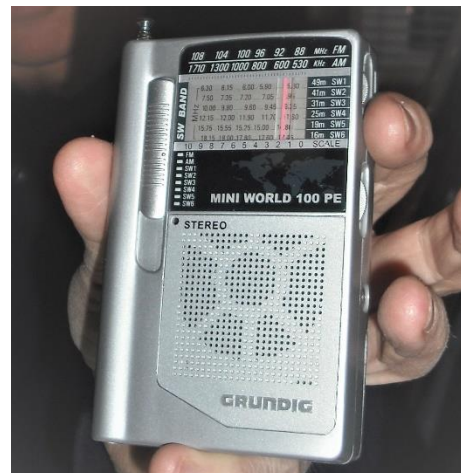
Above & Below: Dave Dean shows his Grundig 100 PE with analog tuning & lots of bandspread on SW bands (next page). This unit from the early 2000's works well and Dave has used in his office. Late Grundig units were made by Eton.
