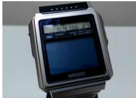
The Guinness Book of Records showed, in its 1984 edition, the SEIKO TV-Watch as the "smallest TV set in the world". This is an interesting theory, since from what you can see here actually looks like the smallest TV by far. Unfortunately, a vital detail is missing; the necessary TV receiver is inside a box about the size of a Walkman.
