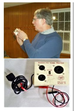
**Above:** Al Simmons shows compact tube tester, the T-110 from the great folks at Fedtro, purveyor of many money saving (read cheap) devices. Why waste your time carrying your tubes to the drug store when you can test any tube with this unit priced under \$10? But it does test for filament continuity with a neon lamp indicator. Al showed some other bargain offerings from Fedtro.
