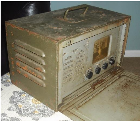
Above: Greg Dottor wonders if better to restore correct color over the clandestine repaint of a Minerva Tropic Master case. Maybe this unit was owned by a perturbed Army serviceman as even the normally unpainted handle has been painted khaki on this normally gray outer case and the painted front cursive lettered logo is gone.
