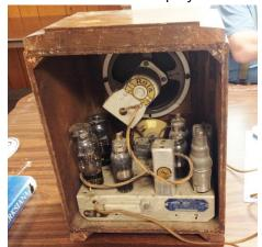
**Above:** Jiri Placek showed a Delco 3201 farm set which employs a robust pair of push-pull 48's in its audio circuit. It was ready to utilize the standard 32 volt DC system often used on farms and also manufactured by Delco **shown below.**
