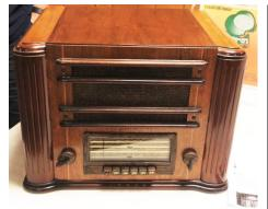
**Above:** Tom Lager showed a 1940 Silvertone 6359 which was value-priced at \$29 to \$35 including the A&B batteries. This was a 6 tube 4 band set employing 1.5 volt tubes and a class B amplifier circuit with AVC. Tom totally refurbished the cabinet and chassis of this beautiful radio.
