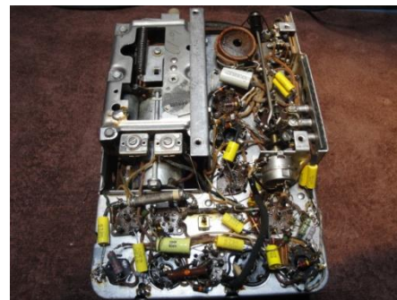
Above: Old caps evident in original state. Below: Lots of replacements and testing, an alignment, and after 3+ hours playing on the bench, I gave the radio my seal of approval.
