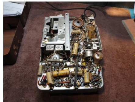
Above: Old caps evident in original state. Below: Lots of replacements and testing, an alignment, and after 3+ hours playing on the bench, I gave the radio my seal of approval.
