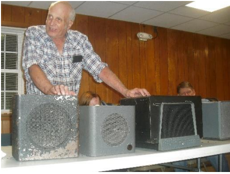
Above: Pete Grave shows off communication receiver speakers. These can be rare since most hams opted out of these pricy accessories relying on their headphones. From left to right, @1949 Hammarlund SC-10 large speaker, RCA speaker from a Canadian model with front control, and Pete's childhood favorite, the Hallicrafters R46 which Pete talked his dad into purchasing for his SX43 rig.
