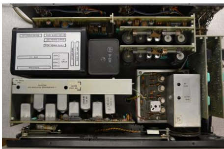
Above: Steve Johnson says Non Linear systems made a FM stereo receiver, the "Modular Stereophonic Receiver 1" for a short period in the late 60's built with a clean modular design like the test equipment they manufactured as their main product line. Below Open Chassis:
