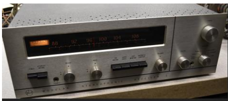
Above: Steve Johnson says Non Linear systems made a FM stereo receiver, the "Modular Stereophonic Receiver 1" for a short period in the late 60's built with a clean modular design like the test equipment they manufactured as their main product line. Below Open Chassis:
