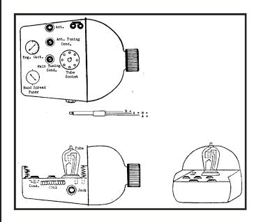
I decided that a reproduction of this historic set would not be too difficult to build. I was surprised that the 12SK7 fit across the narrow dimension of thecanteen. I used a straight-forward regen circuit with a tapped coil and antenna coupling via a trimmer cap. It tunes about 5 to 12 MHz. A circuit of this sort will work with as little as 12 volts on the plate. The standard canteen cup covers the opening when it's in the cover. When you pick it up it just feels like a
