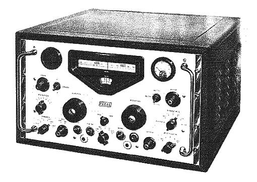
to 30.5 MHz in 30 1-MHz bands. Through a high degree of mechanical and electrical complexity, and a few annoying compromises, it accomplishes this with only 10 crystals.
