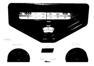
The RA.17 occupies 10 3/4 inches of rack space, which was pretty much standard communication receiver size in this era. The diecast aluminum chassis pushes the weight to 67 pounds versus 43 for the 51J. The receiver uses 22 miniature tubes plus a rectifer. The commonly available "C" models use US tubes. Tuning range is 0.5 to 30 MHz in 30 1-MHz bands. The approximately \$1000 introductory price crept up to \$2400 before production ended.
